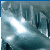
■ Cutting edge after 1.000 holes tapping
