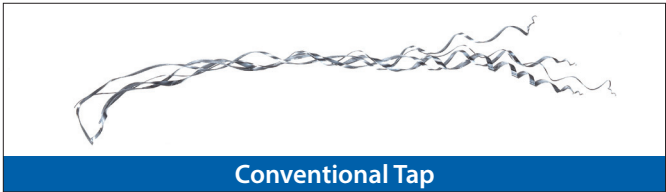
■ Chip generated in 40m/min
